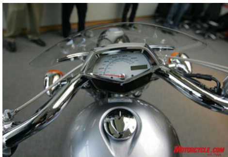
Internally wired bars and a clean instrument panel offer both style and function. Seen here is an optional windscreen, just part of a large selection of Fury accessories in Honda's catalog.
