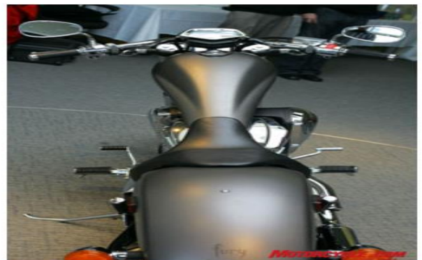
While the fuel tank on the lean Fury is eye catching, it does come at a cost as it only holds a modest 3.4 gallons.
