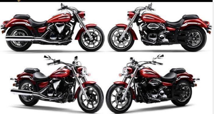
**Specifications:** Engine: 942cc, liquid-cooled, fuel-injected, 4-stroke, 4-valve, OHC V-twin
